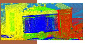
3D point cloud shall be converted to mesh model in order to prepare sections and coordinates for precise accuracy MOCE
